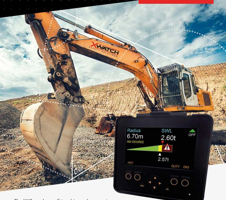
The XW2 can be configured to work on any type of hydraulic excavator. Overload and height limitation is controlled using proportional soft-stop hydraulic valves providing accurate and repeatable performance without detriment to the machine. A basic dig depth monitor is available when the RCI is not required. If hazards arise, XW2 will automatically flip to the relevant display page.
