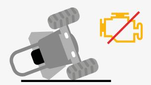
In its standard guise, maximum roll angle can be set from 1 to 32 degrees (0- 63%). An audible alarm sounds when the maximum tilt has been exceeded. Intelligent filtering is used to separate actual machine tilt from bouncing and vibration. In the unfortunate event of a roll-over SS2 will send a signal that can be used to cut the engine, and/or activate a siren or beacon.
